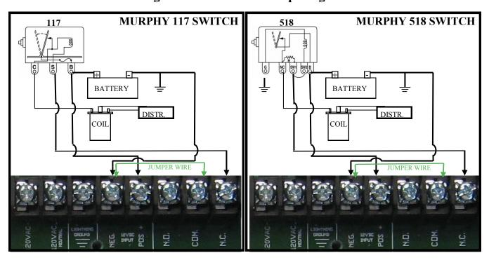
**CAUTION**: Never switch any voltage greater than 120v with the Hot Shot Receivers internal relays. This will ruin the relay and void all manufacturer warranties. Use an externally mounted 120v coil relay to switch all voltages greater than 120v. See diagram on next page.
